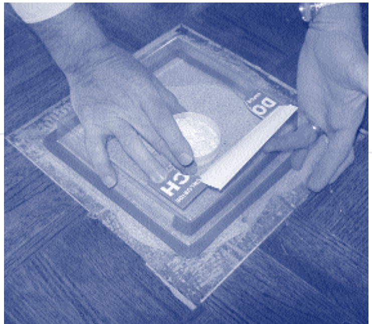
Calcium Chloride Test being retrieved after 64 hours of moisture testing.
